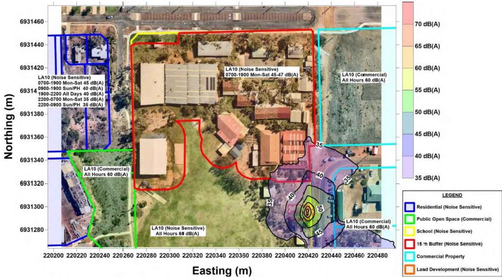
Figure 4 - A-weighted SPL Contour Plot for Kalbarri District High School BESS at proposed location, without noise mitigation panels installed.
