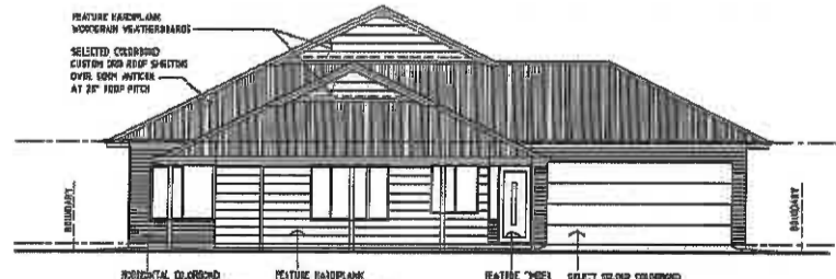
NORTH ELEVATION 1:100 (STREET VIEW)
