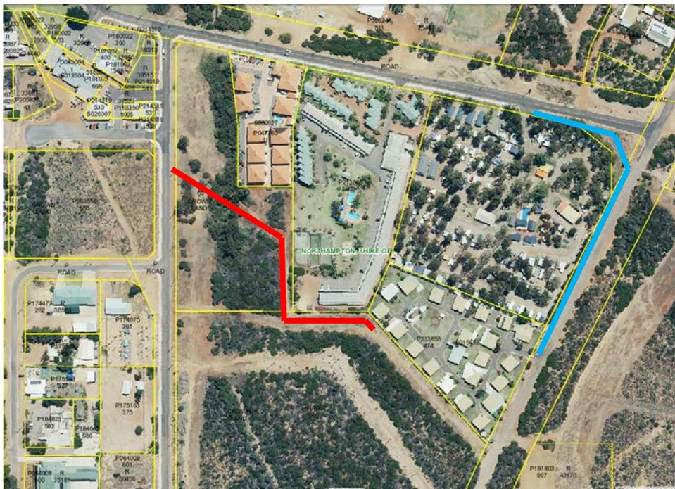
Option 1 has a number of issues in relation to the control and avoiding of a major drainage area at the intersection of Porter and Nanda which will require installation of culverts etc.
